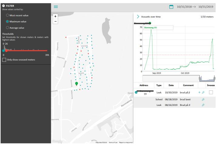
In this particular district they found a lot of leaks, due to the pipes being installed in the 50's. The leakage in this district dropped from  $1,7m^3/h$  to 0,3  $m^3/h$ .
